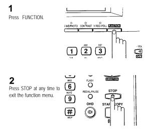
✓ If you press a button while the LCD is cycling through the function menu, the machine assumes you want to change the function setting corresponding to that button choice.
